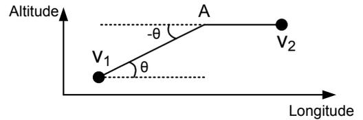
Figure 2: Altitude-longitude Projection of a Road Segment
