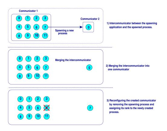
Figure 1. Steps involved in communicator handling to achieve MPI process migration.
