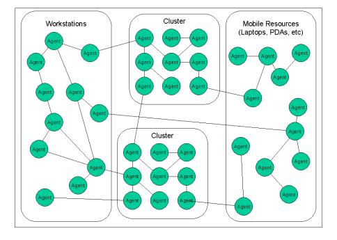
Figure 4. The peer-to-peer virtual network topology. Middleware agents represent heterogeneous nodes, and communicates with groups or peer agents. Information is propagated through the virtual network via these communication links.
